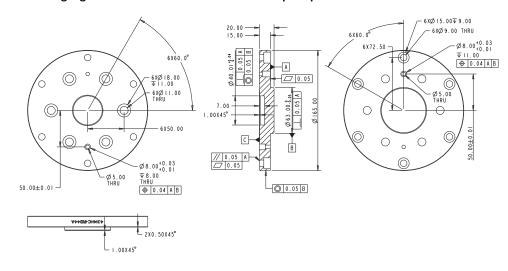
Following figure shows the dimension of adapter plate M4.
